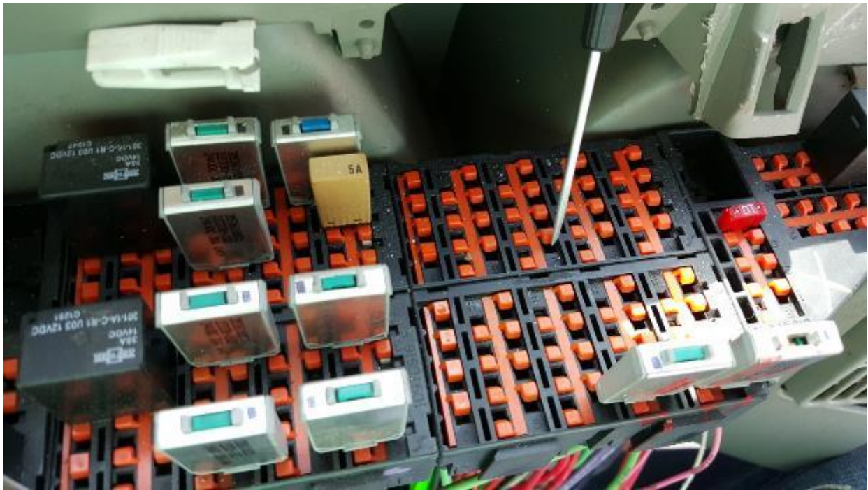
a) Prostar/Workstar/DuraStar/TransStar Pin location for constant power:
