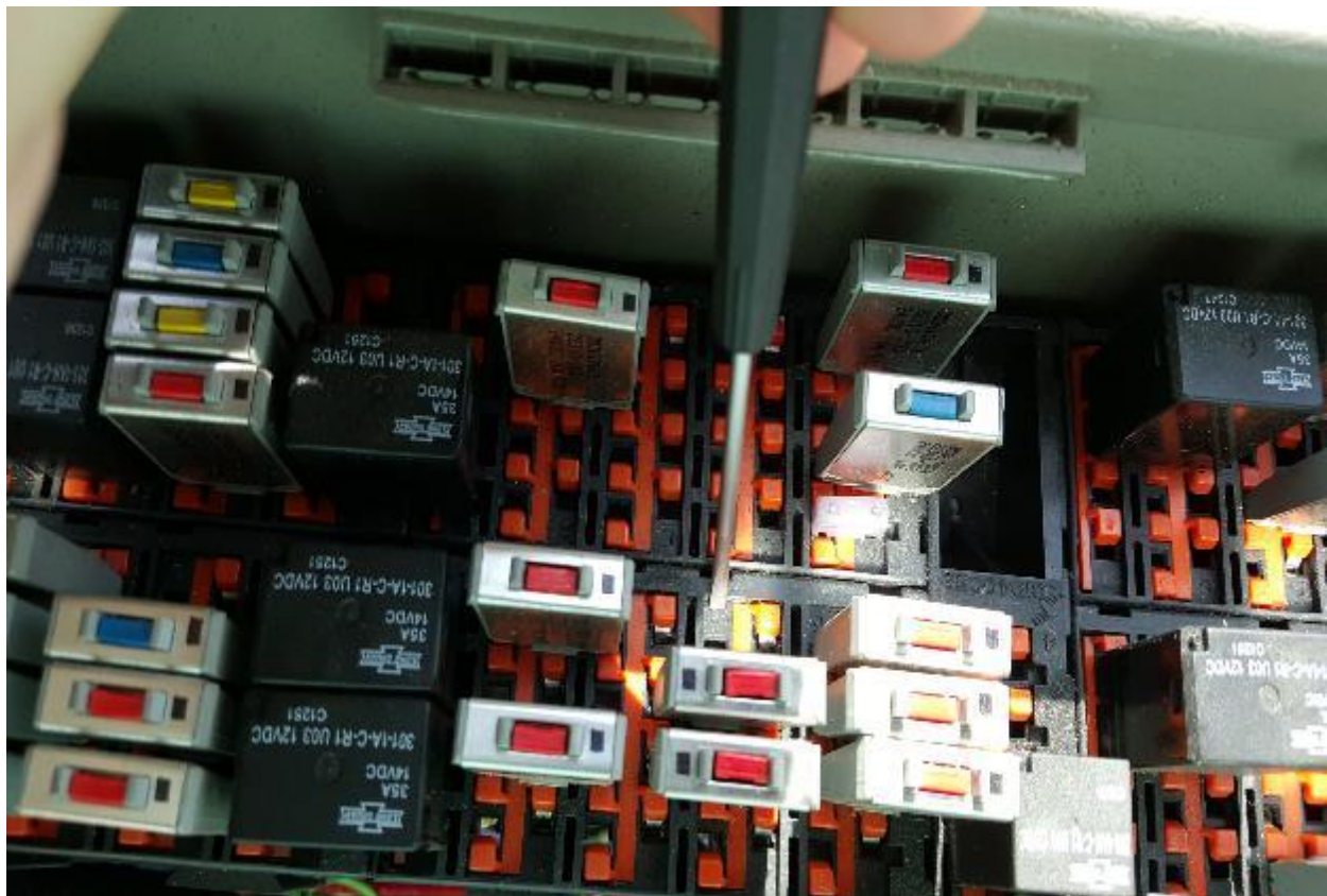
b) Prostar/Workstar/DuraStar/TransStar Pin location for Ignition:
